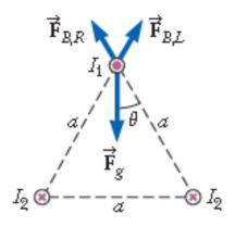
$$I_2 = \frac{(0.400kg)(9.80m/s^2)\pi(0.0100m)}{(4\pi \times 10^{-7}T \cdot m/A)(100A)(10.0m)\cos 30.0^{\circ}}$$
