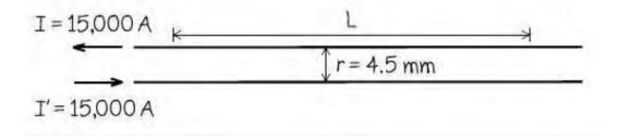
$$\frac{F}{L} = \frac{\mu_o I_1 I_2}{2\pi r} = \frac{4\pi \times 10^{-7} \times 15000^2}{2\pi \times 4.5 \times 10^{-3}} = 1 \times 10^4 \, N/m$$
